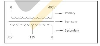
7.4 NDK-100, capacity: 100VA, input 400V, output 36V
