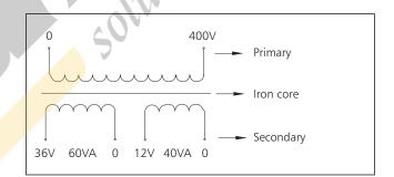
7.3 NDK-100, capacity: 100VA, input 400V, output 36V 12V
