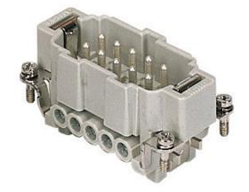
Male insert, CNE series, screw terminal connection, 10 poles + PE, 16 A 500 V 6 kV 3, size "57.27", with plate
