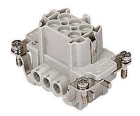
Female insert, CNE series, screw terminal connection, 6 poles + PE, 16 A 500 V 6 kV 3, size "44.27", with plate
